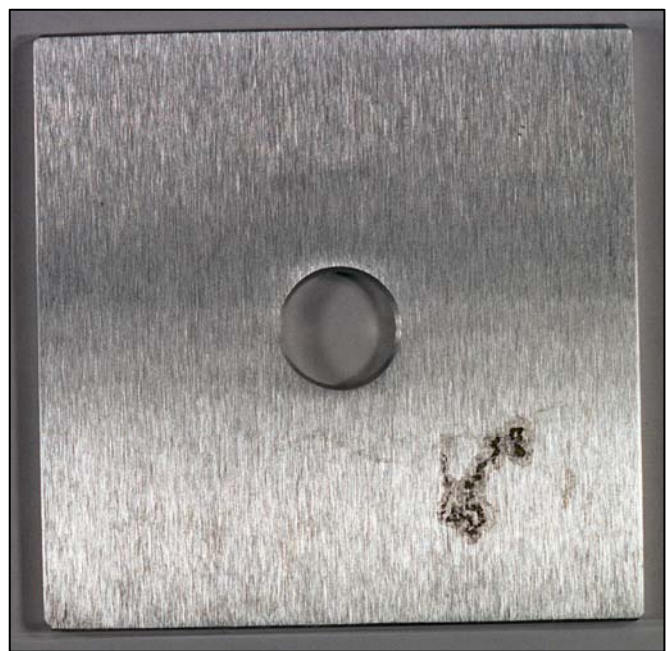
FIGURE 8 - Aluminum Coupon After Cleaning, 6-year exposure at 3.05-m
