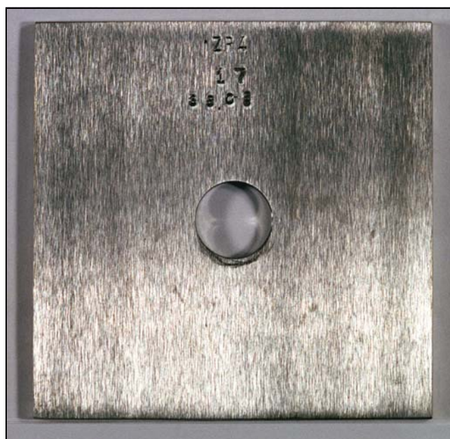
FIGURE 1 – Zirconium Alloy Before Cleaning, 6-year exposure at 1.22 m
