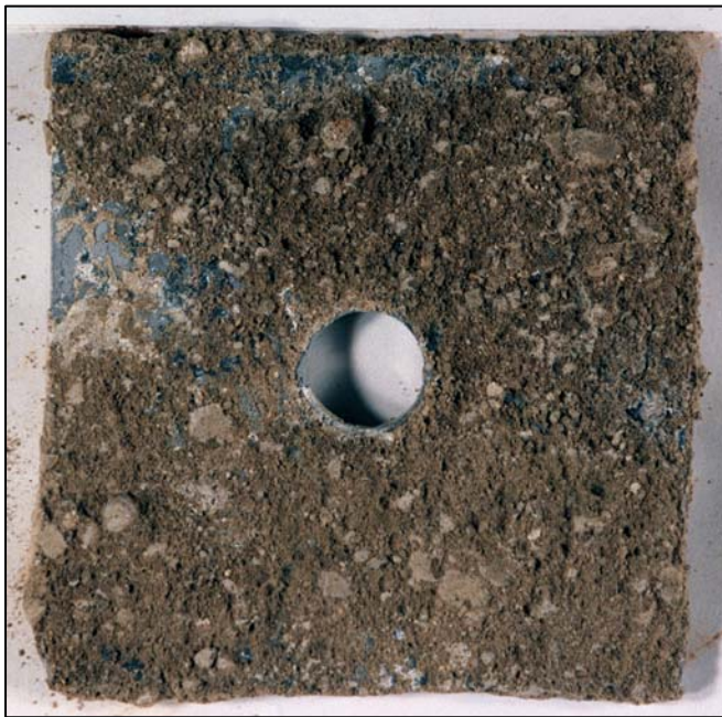
FIGURE 5 - Beryllium Coupon Before Cleaning, 6-year exposure at 3.05-m
