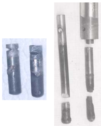
Fig. 3. Be Samples Be5, Be6, Be9 and Be10 (left to right) exposed for 150 hours at 530°C in molten flibe.
