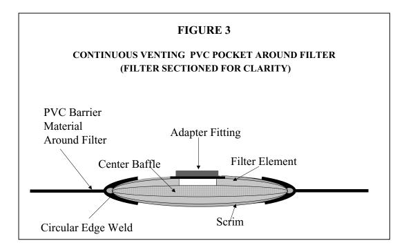
Other methods are being developed for sealing to PVC and polyurethane that would improve the durability of the filter mounting. A similar pocketing technique identified in Figure 4 can be made airtight by sealing the barrier material to the flange of the adapter fitting. Special fittings or tape can cover the outlet of the adapter fitting to seal the bag.
