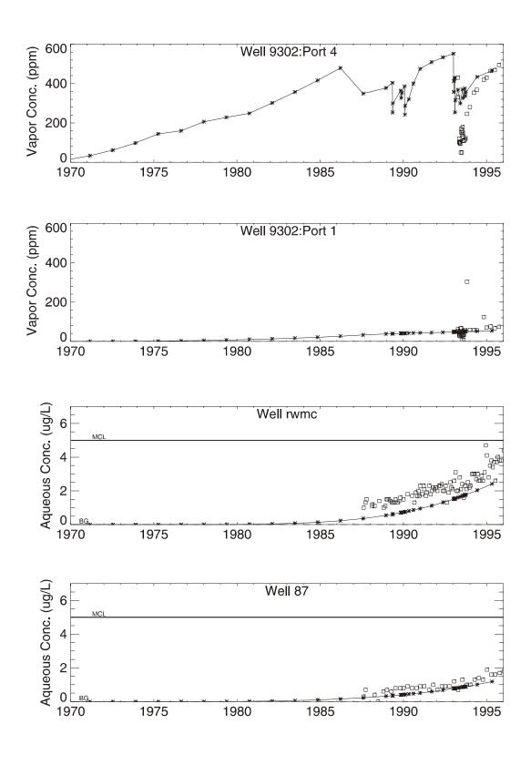
**Figure 4.** Simulated (asterisks) and measured (boxes) CCl4 vadose zone vapor and aquifer concentrations.
