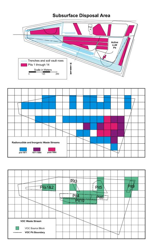
**Figure 3.** Subsurface disposal area and assignment of contaminant source releases for simulations.
