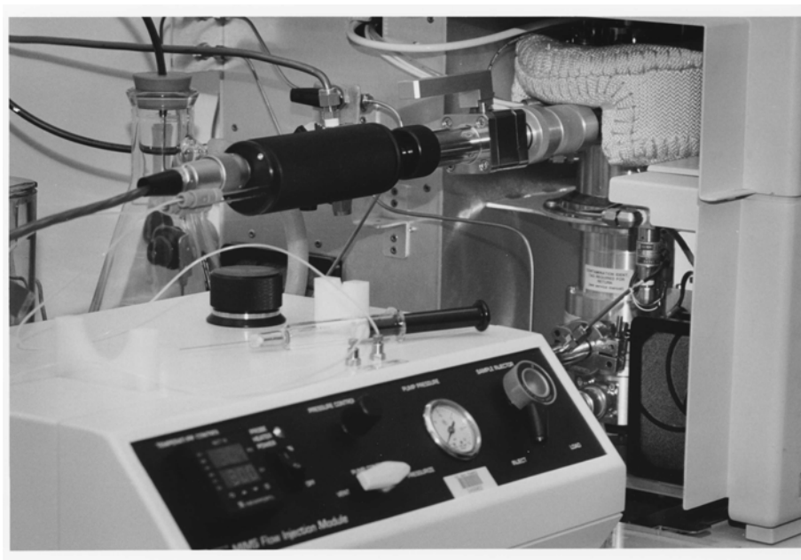
Figure 13. Close up view of the probe that has been inserted into the side of the mass spectrometer.
