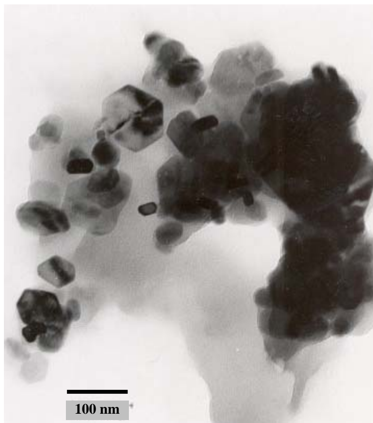
Figure 2. TEM micrograph of CuS nanoplatelets.
