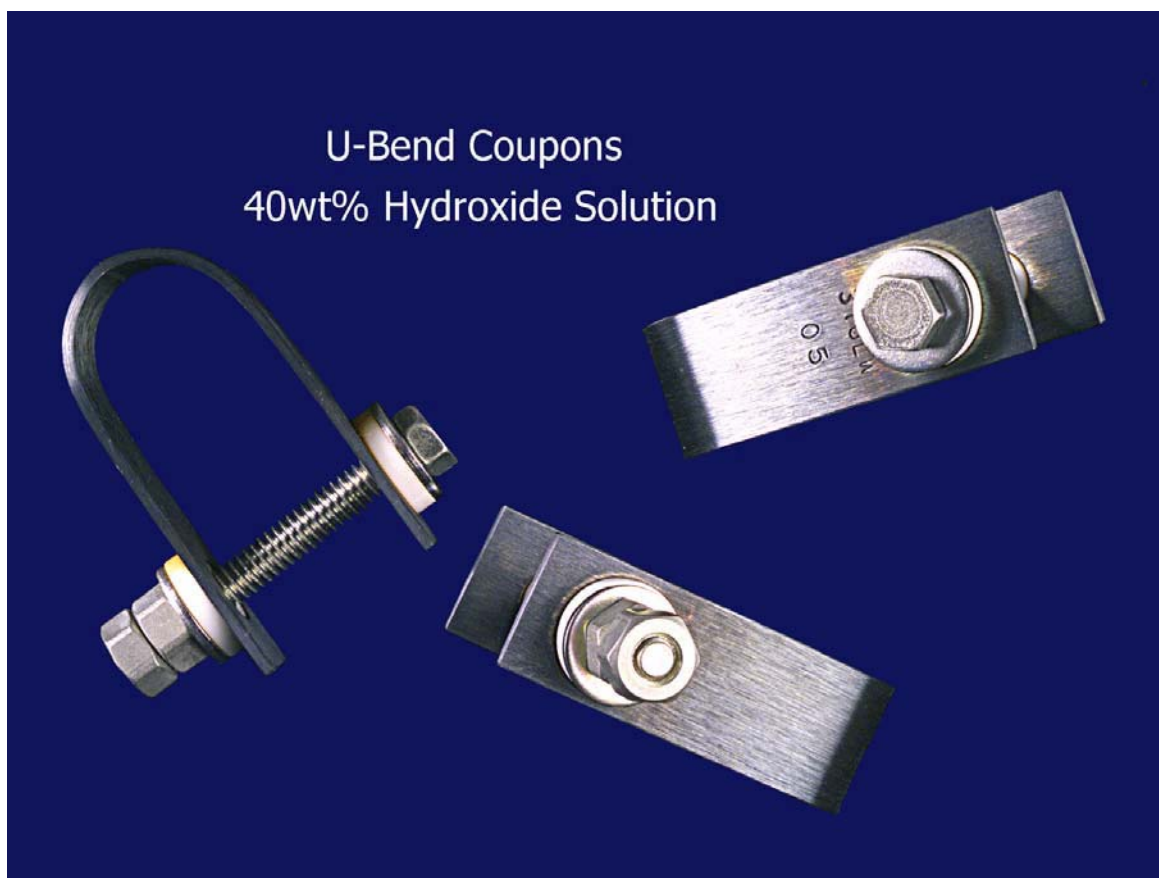
Figure 8. Type 316LW tested in 40-wt% hydroxide solution with halides at 90°C.
