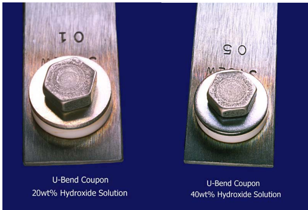
Figure 7. Type 316LW U-bend coupons showing liquid/vapor interface area.
