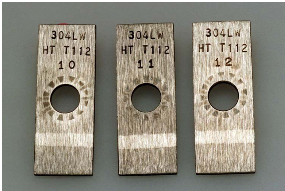
Figure 13. Type 304LW tested in 20-wt% hydroxide with halides at 90°C.
