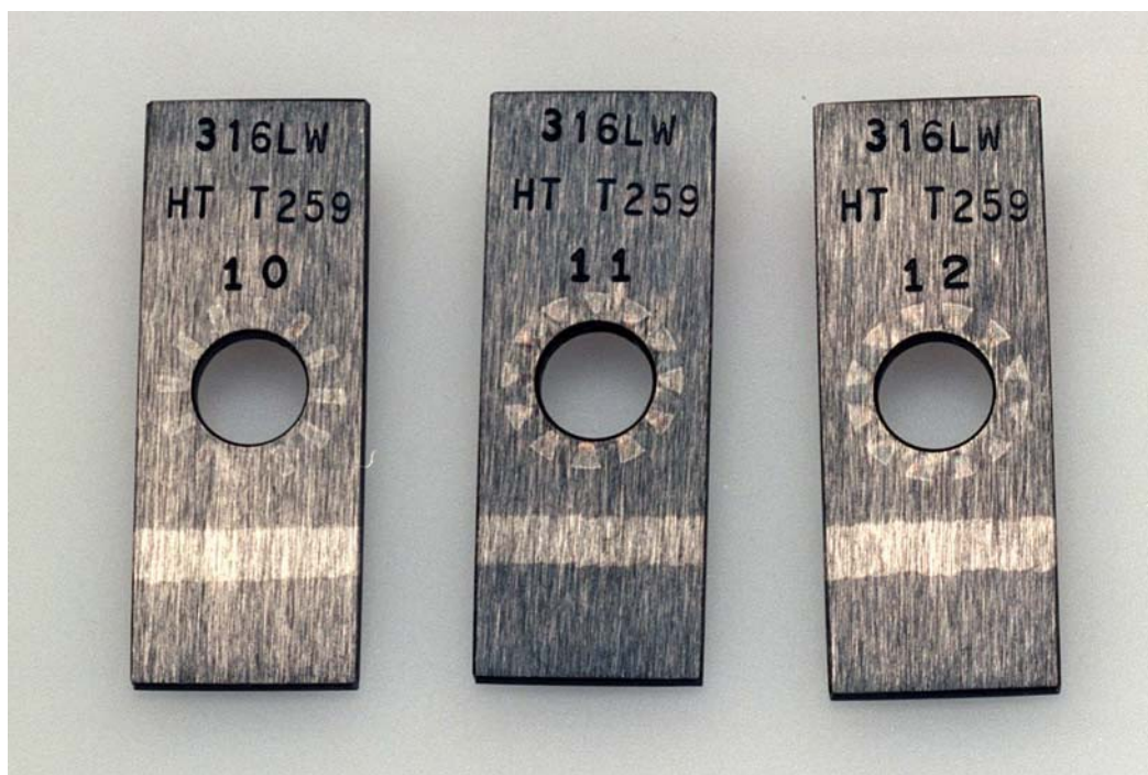
Figure 4. Type 316LW tested in 40-wt% hydroxide solution without halides at 90°C.
