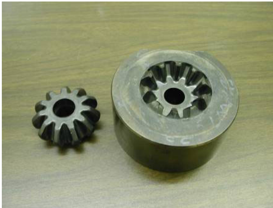
Figure 43. Spray-formed M2 tool steel forging die with forged steel gear.
