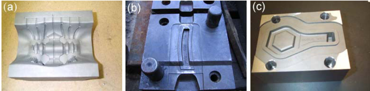
Figure 72. Die inserts manufactured on the commercial RSP tooling machine. (a) P20 injection mold insert. (b), (c) H13 forging die inserts.
