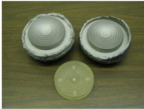
Figure 45. As-deposited A2 tool steel glass-forming dies and stereolithography master.
