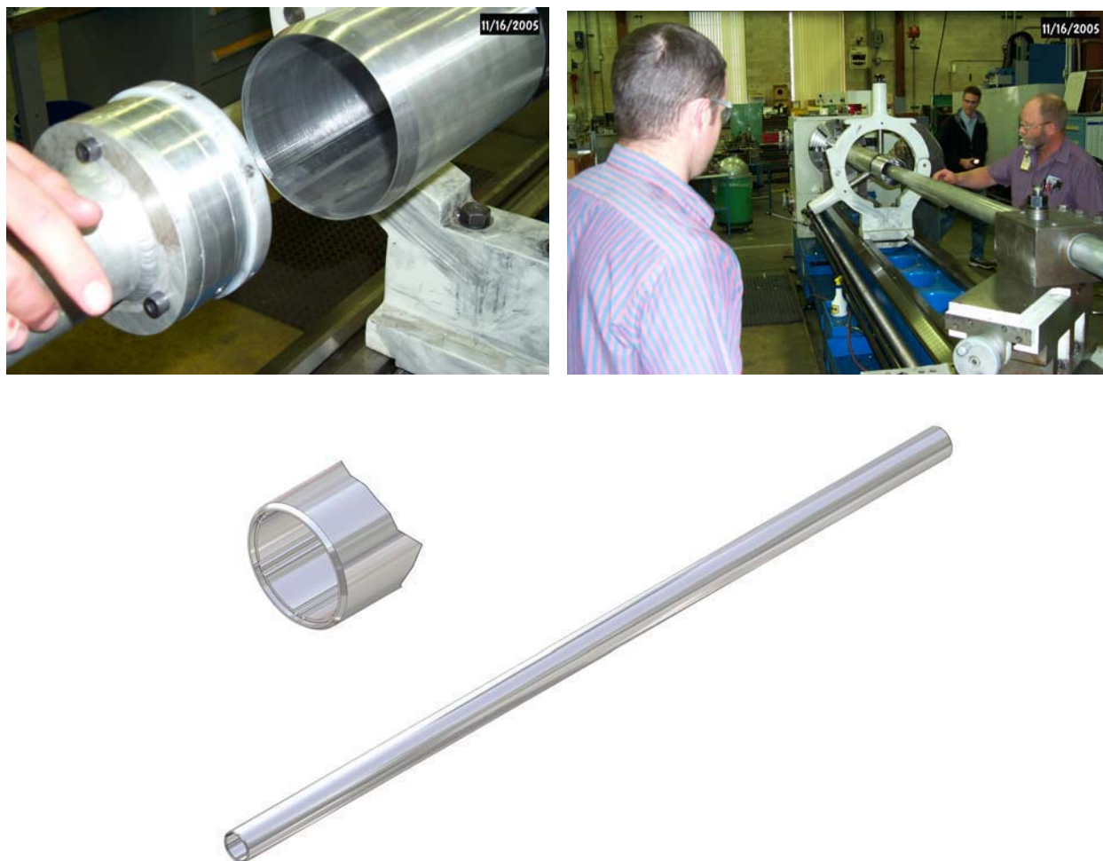
Figure 25a, b, and c. Grooved AGC-1 pressure boundary and broaching operation at the ATR machine shop
