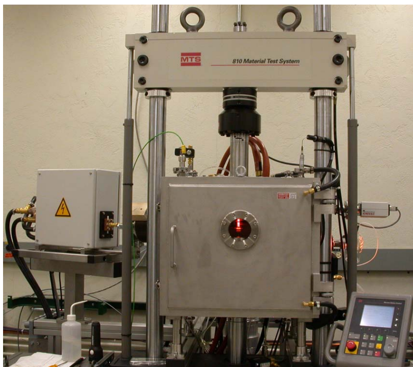
Figure 44. Environmental chamber installed on creep-fatigue load frame.
