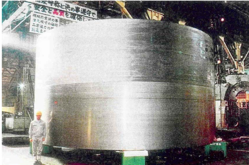
Figure 22. ABWR RPV beltline forging of ASME SA508 (127 tons, 7.48m OD, 7.12m ID, 3.96m high) [31] .
