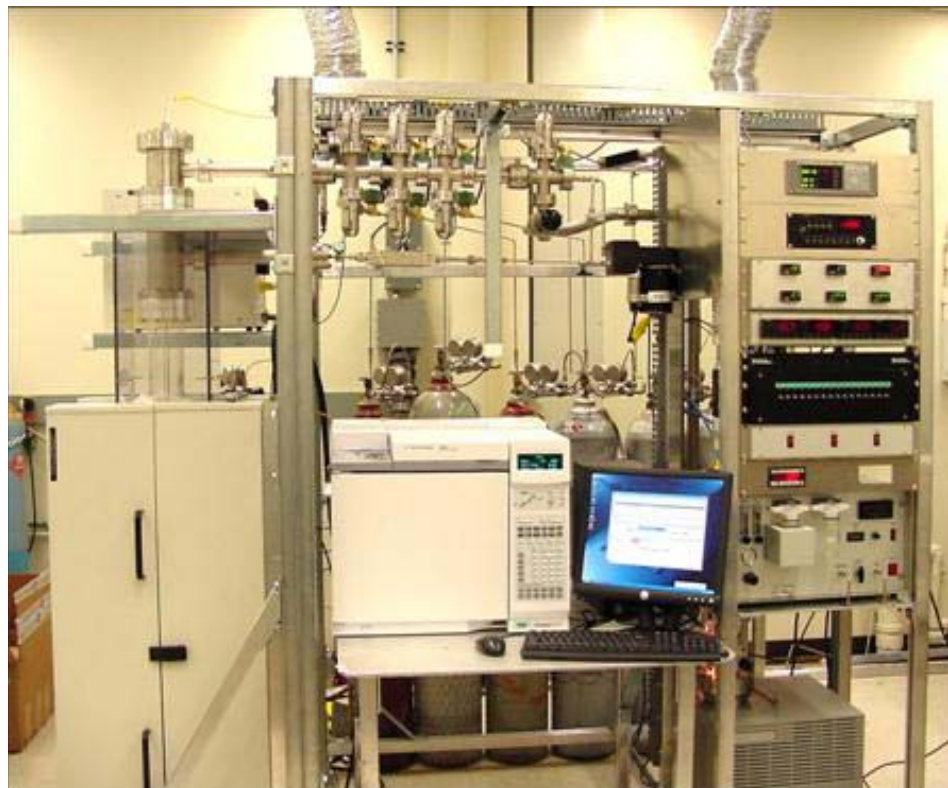
Figure 45. Photograph of the assembled low velocity controlled chemistry test loop.
