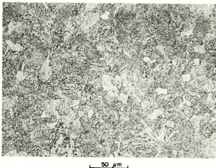
Figure 23. Optical photomicrograph of SA 533B steel, quenched and tempered: upper bainite and granular bainite with grain size of ASMT 8-9 [32]
