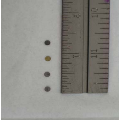
Figure 2.14. Sample disks for micro-hardness tests.
