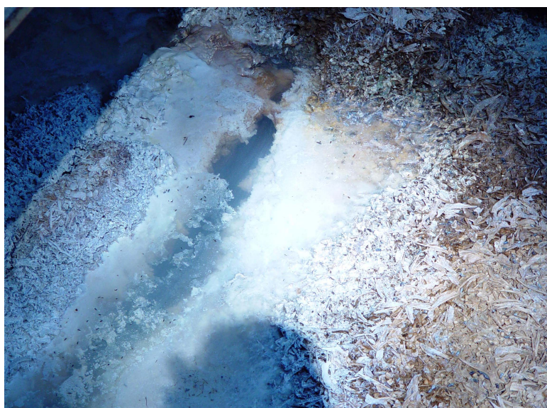
Figure 9. Sediment buildup in the Reactive Media.
