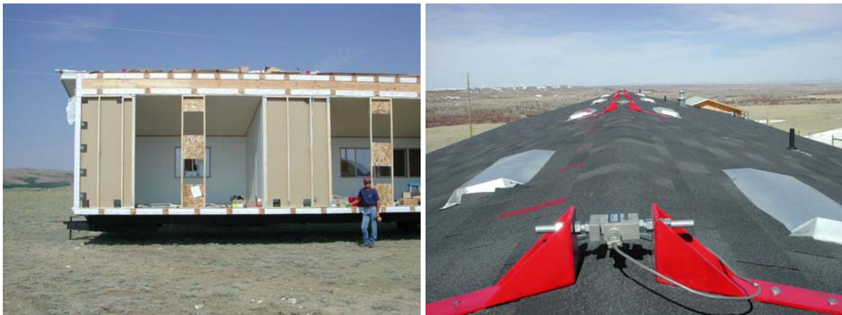
Figure 3. Installation of marriage line load cells on floors, exterior walls, ceiling, and roof
