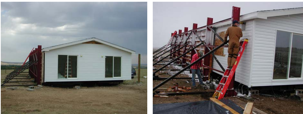
Figure 1. Double-wide test home simulated lateral load tests
