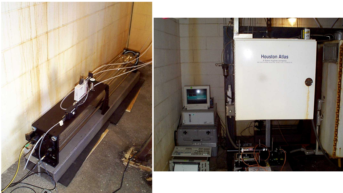
Figure 24. Multi-pass cell (left) and near-infrared spectroscopy instrumentation (right) deployed behind Houston Atlas system at NCPA Unit 1.
