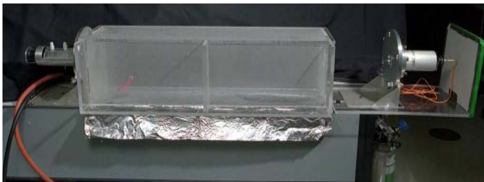
Figure 5. Photograph of experimental setup for condensate measurements.
