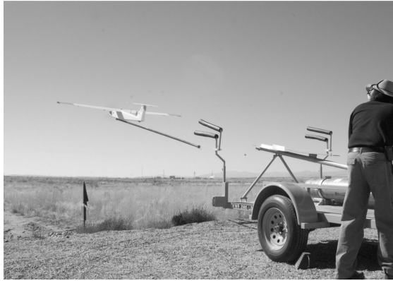
Fig 1. Autonomous Catapult Launch of First Responder UAV
