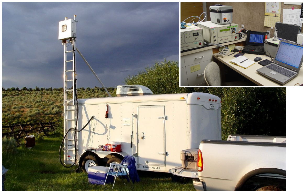
Figure 2. INL Mobile Hg Monitoring Lab with Tekran® instrumentation (1130 quartz denuder module shown on 4-m high tower).
