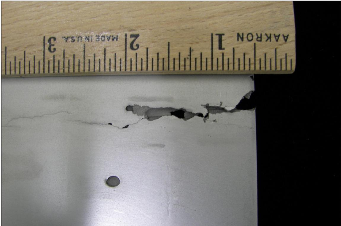
FIGURE 3. Sensitized Type 304 with Evidence of Pitting,, Cracking, Penetration, and Tunneling.
