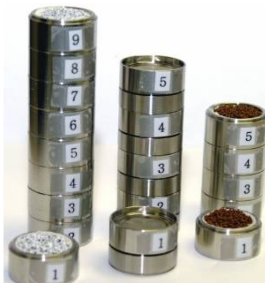
Fig. 2. Filter media for DEOX testing includes zeolite (center) and aluminosilicate (left, right) based materials.
