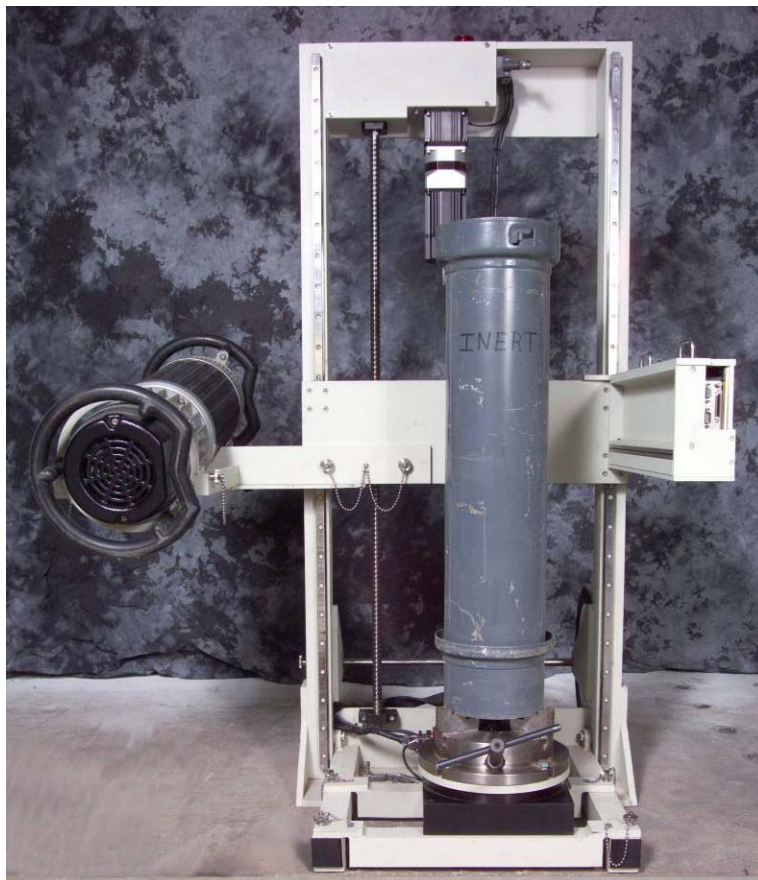
Figure 1-3. DRCT Gantry with x-ray generator, detector, and rotational stage installed.
