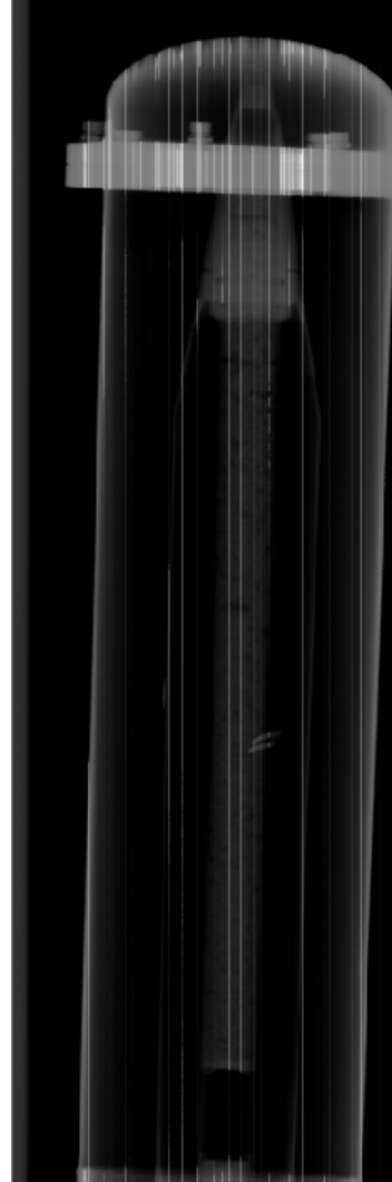
Figure D-2. Improperly calibrated detector image.
