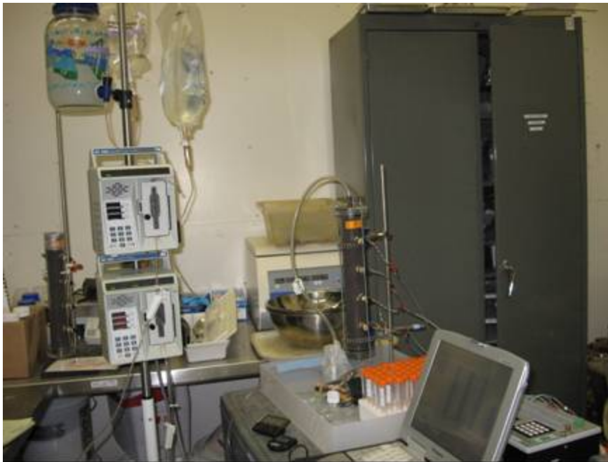
Figure 2. Experimental set-up for 1D column polymer tests.
