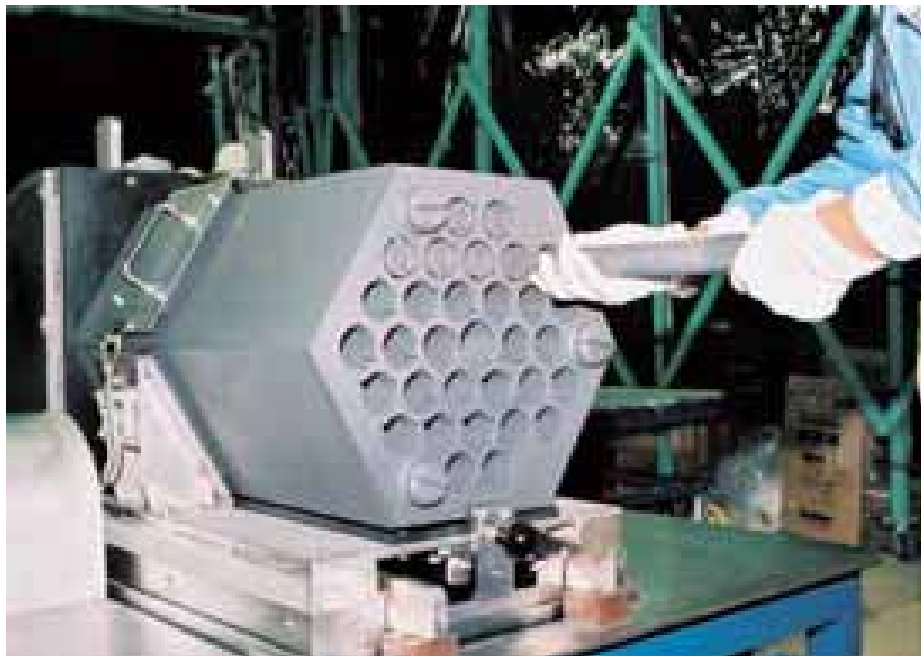
Figure 1.55. Assembly of a Fuel Element Block. a
