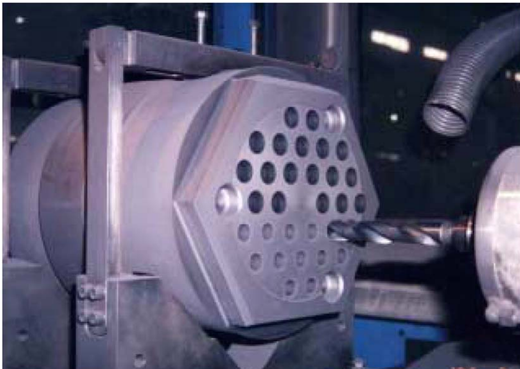
Figure 1.82. HTTR Graphite Block Undergoing Machining. a
