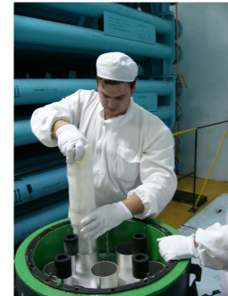
Figure 2: Loading IRT-2M HEU into Casks
