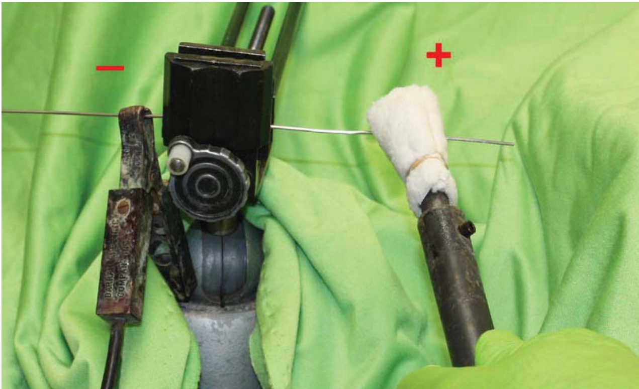
Fig. 3. Cleaning of surface of refractory lead to be brazed. Tool on the right consists of a graphite-tipped electrode covered with a cotton sock that had been soaked in sulfuric acid/ammonium sulfate solution. The refractory metal surface was scrubbed until the sock wiped clean.
