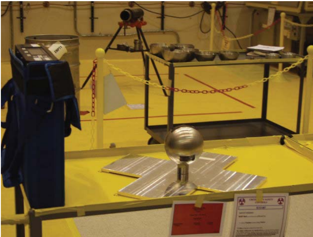
Fig. 2. Photograph of the Plutonium Sphere with 1.27-cm-Thick Nickel Reflector using the Feynman Method.
