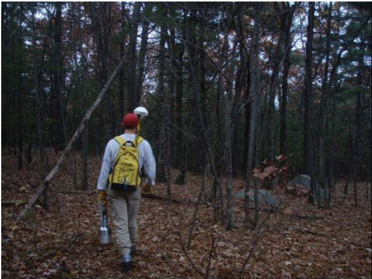
Figure 3. BaSIS system and operator conducting radiation survey at Shepley's Hill site. Note: The radiation detector is to the left of operator.
