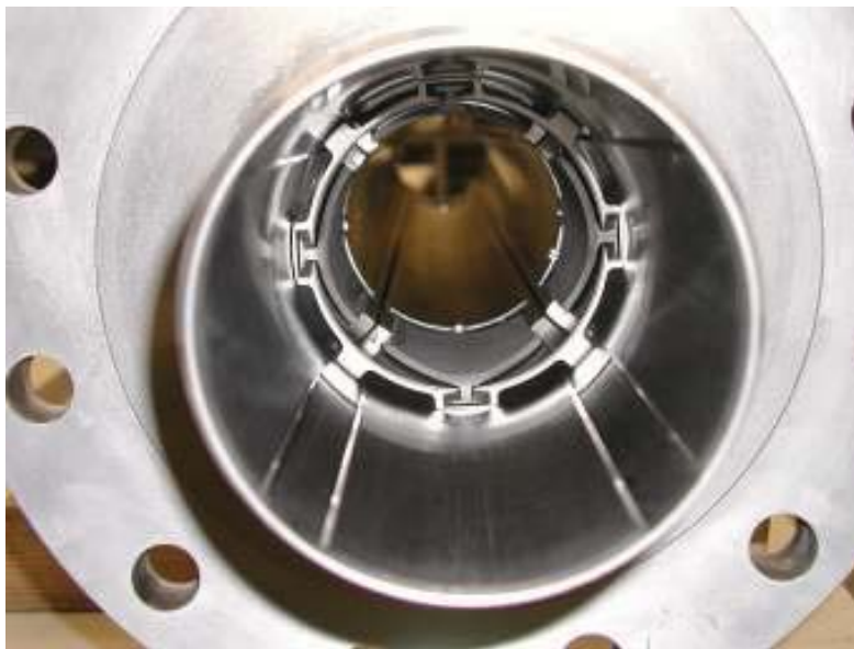
Figure 11. View of the lower support ring in the model flow baffle assembly from below with the model booster fuel elements installed.
