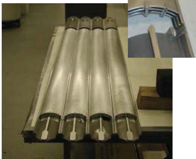
Figure 10. Model booster fuel assemblies. The second from the left has brackets (inset) to hold the Pitot tubes used to measure flow velocities.
