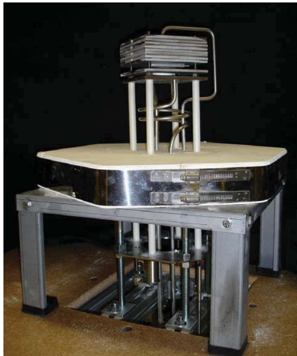
Figure 4-5. Test stand installed in furnace base.
