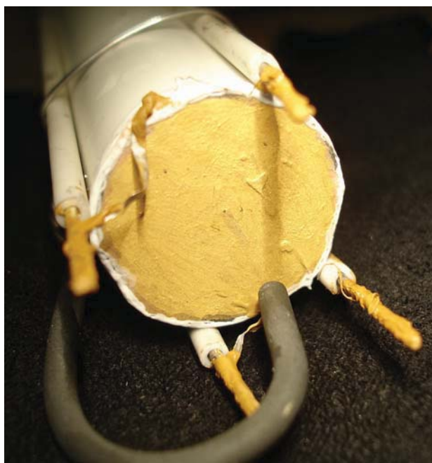
Figure 5-2. NASA button cell mounted on support tube.
