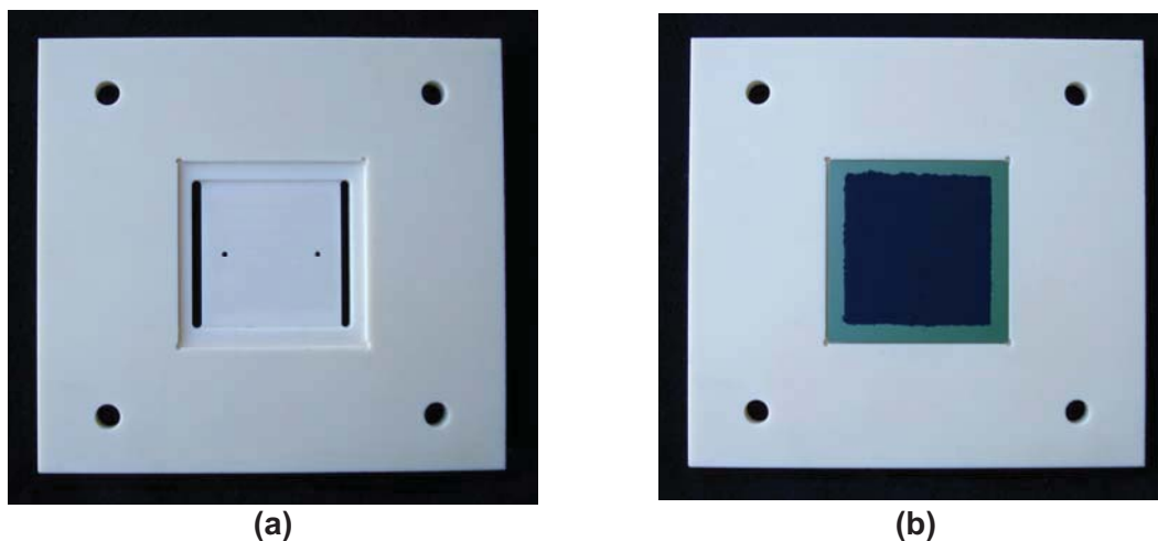
Figure 4-2. (a) alumina cell holder; (b) cell holder with cell in place.
