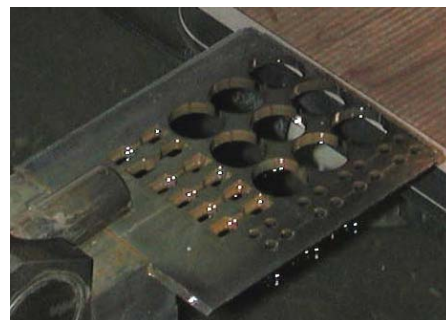
Figure 35. Photo showing the locations where specimens were EDM machined from a plate cut from the ACO-3 duct.
