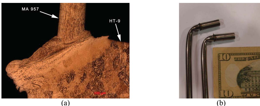
Figure 45. (a) An optical micrograph of the PRW joint cross-section. (b) Two bend-tested samples of the cladding tube - plug PRW joints.
