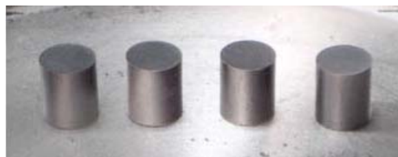
Figure 4. Pellets of four different MOX and MA-MOX compositions fabricated using the simplified process.
