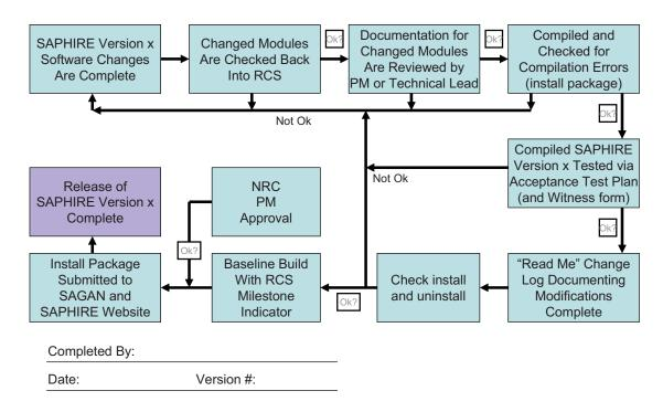
Figure 1. SAPHIRE release management process.
