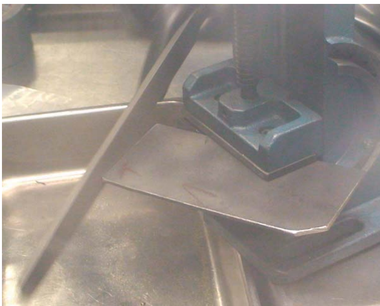
Figure 6. Edge filing of a UMo coupon in an argon atmosphere glove box.
