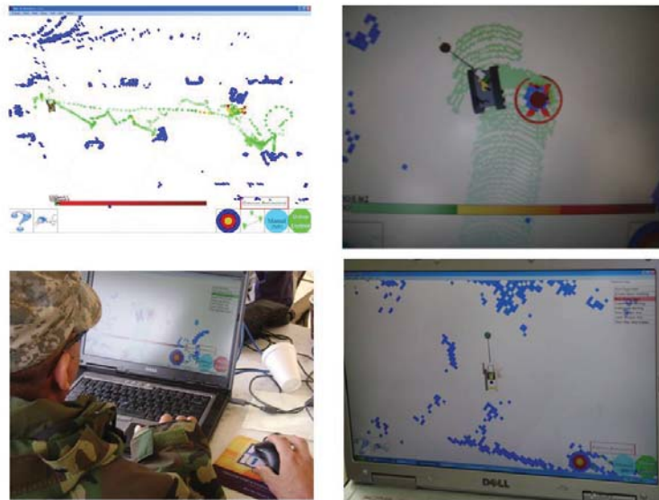
Figure 4 Screen shot of the OCU during different missions, showing control of the robot using a tasking target with waypoints, hazard map, and sensor readings. (SHOULD BE ENLARGED A LITTLE BIT AND ANNOTATED)
