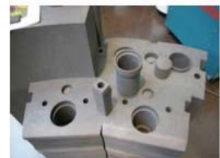
Figure A-2. Graphite core components.
