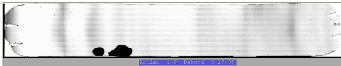
Figure 1. An example UT scan that was produced for an annealing study fuel plate.
