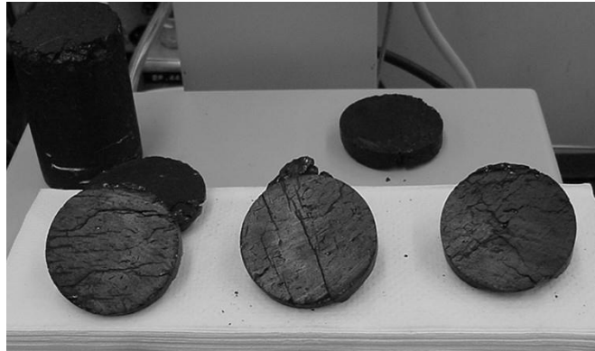
Figure 6. Photograph of trimmed ends from Gilson-seam coal cores 2 in. in diameter. Note the irregular cleat system associated with this coal.
