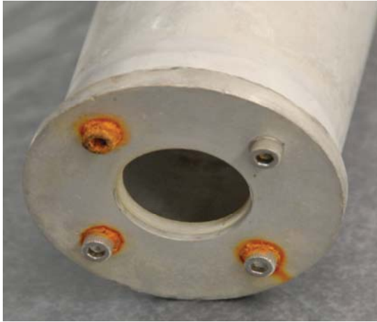
Figure 7. Corroded Fasteners on Shim Rod #2 Barrel
