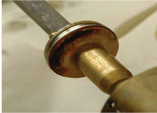
Figure 8. Corrosion on Shim Rod #2 Piston
