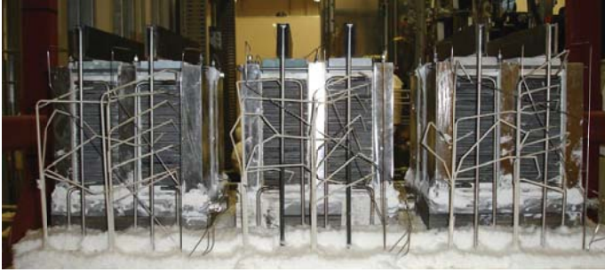
Figure 16. ILS hot zone with three HTE modules installed.
