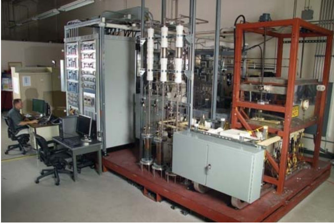
Figure 13. 15 kW Integrated Laboratory Scale HTE test facility at INL.
