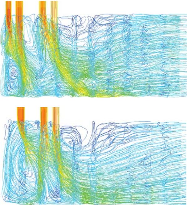
Figure 7. Streamline plot for SKW model for four-jet (upper) case and three-jet case.
