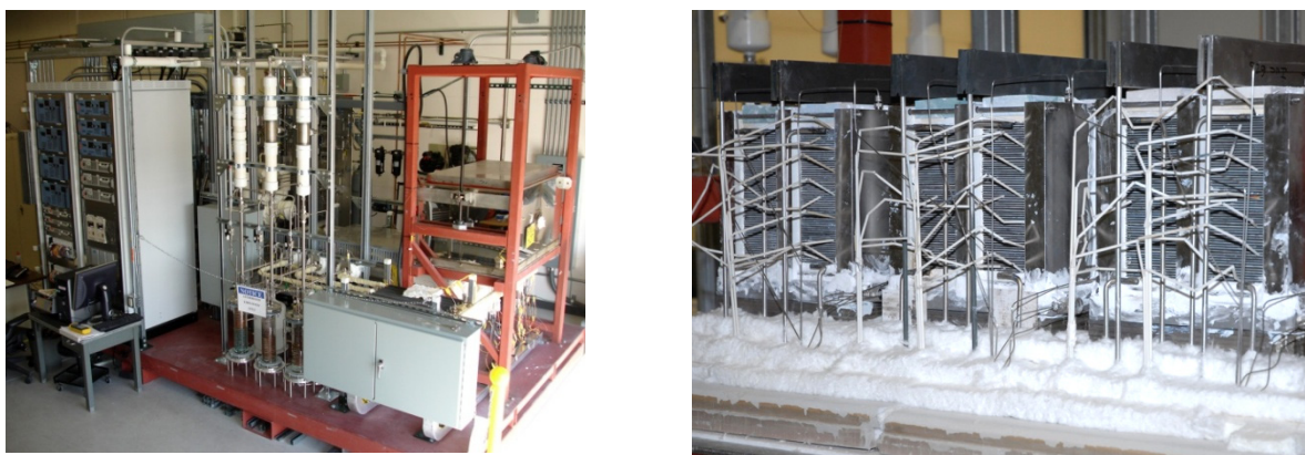
Figure 25. HTE integrated lab-scale experiment (left) and three electrolytic modules (right).
