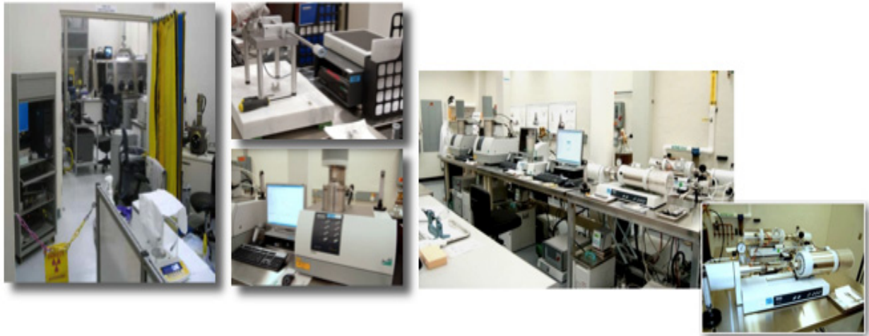
Figure 8. Graphite characterization laboratories - showing thermal and physical characterization equipment such as Laser Flash Diffusivity, thermal dilatometer (CTE measurements), Thermal Gravimetric Analysis (TGA), and ultrasonic physical measurement equipment.
