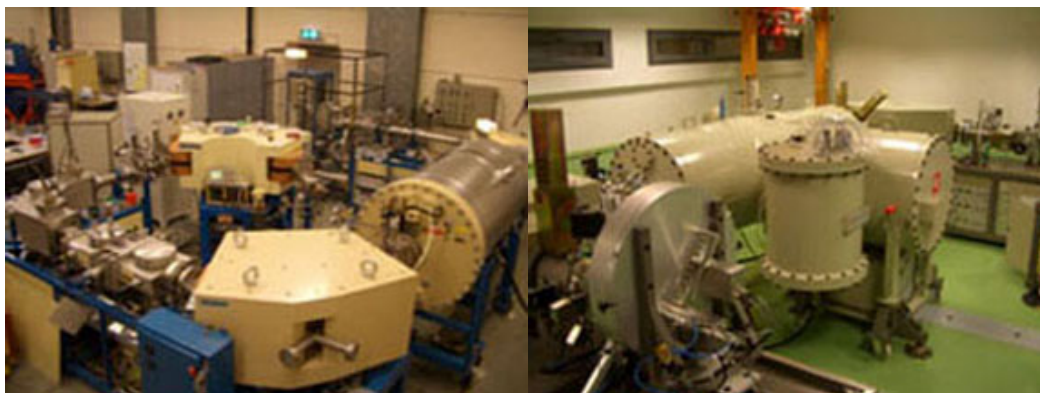
Figure 2. Left, NEC 0.5 MV AMS system at ETH in Zurich. Accelerator tank on right of photo. There is an extraneous magnet, un-needed for iodine analyses, at center of image. Right, HVEE 1.0 MV AMS system at CNA in Seville. Sample wheel assembly at lower left.
