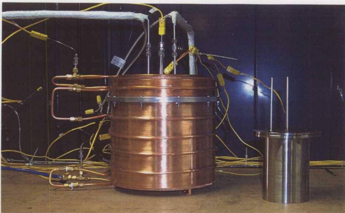
Figure 8. Preliminary test setup for Molten-salt Safety Experiment.
