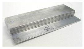
FIGURE 1. Stack of aluminum plates joined by friction stir welding.
