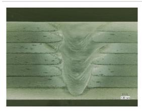
FIGURE 3. Cross-section of the stack of aluminum plates joined by friction stir welding shown prior to machining the solid bar from the center of the above stack.
