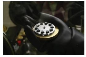
FIGURE 3. TRU-MOX pellets fabricated in the AFCI glove
