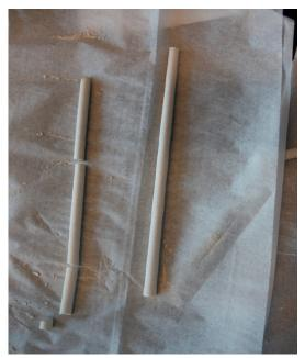
FIGURE 1. Dry Bag Isostatically pressed rods comprised of CeO<sub>2</sub>
