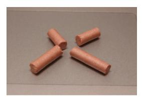
FIGURE 2. Densified  $CeO_2$  rod pieces after sintering in a high temperature furnace.
