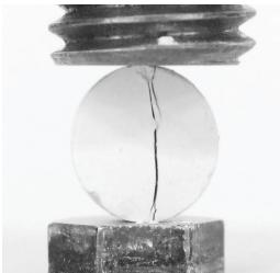
FIGURE 4. Diametral strength testing of a green pellet.
