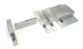
FIGURE 2. Stack of aluminum plates section for examination. A solid bar of aluminum is marked  $A \leftarrow B$  in the photograph.
