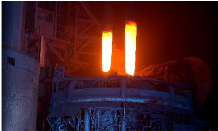
Figure 12. Graphite electrodes being inserted into a scrap metal furnace.
