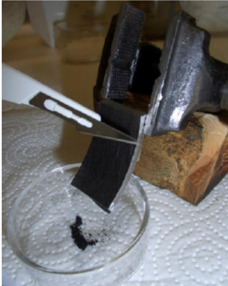
Figure 10. Removal of dust by scraping a section of AVR pipe (Fachinger et al. 2008).
