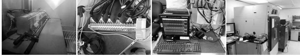
Figure 1 Test equipment and Tenney Chamber (from left to right, Moore modules, sensor terminal block, Honeywell recorder, Tenney Chamber)
