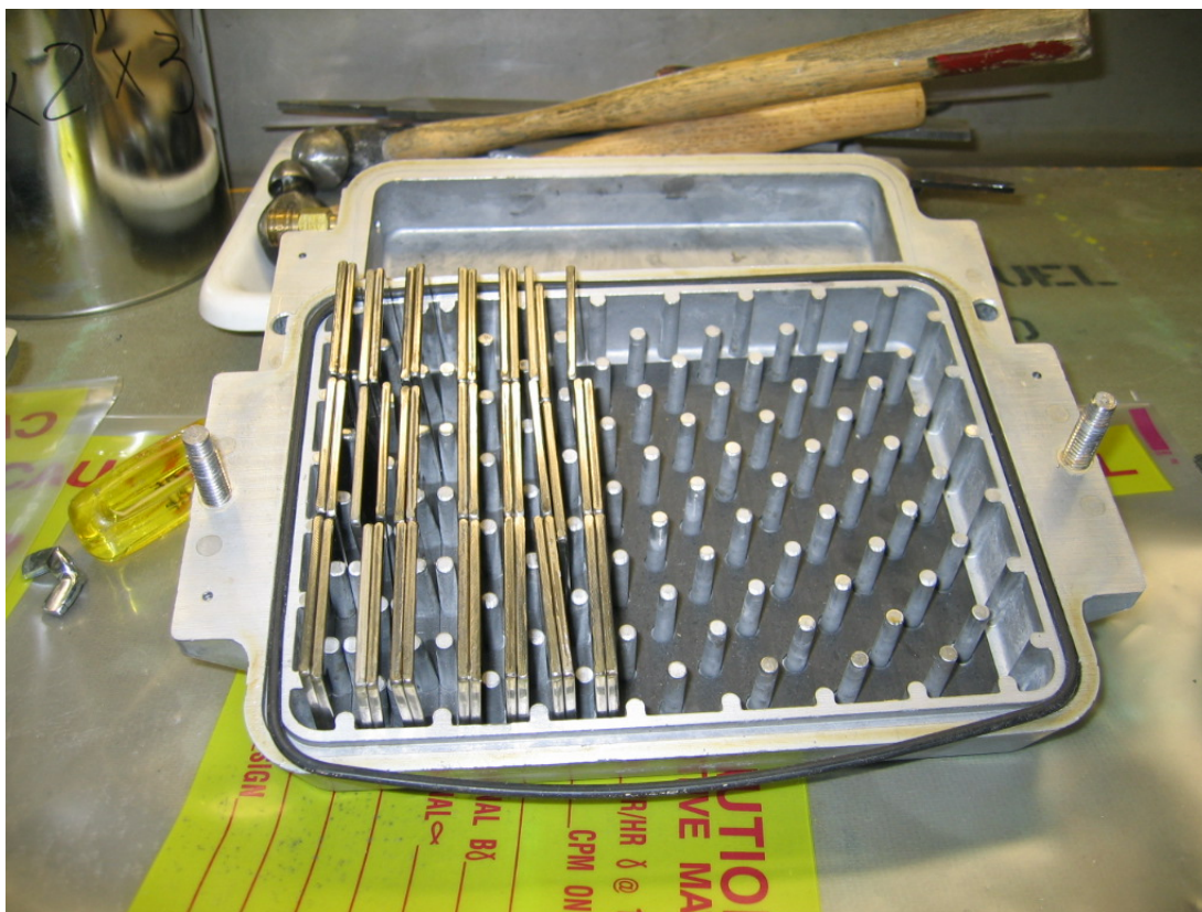
Figure 4. A representative ZPPR fuel-plate clamshell (partially filled with PuAl fuel plates).
