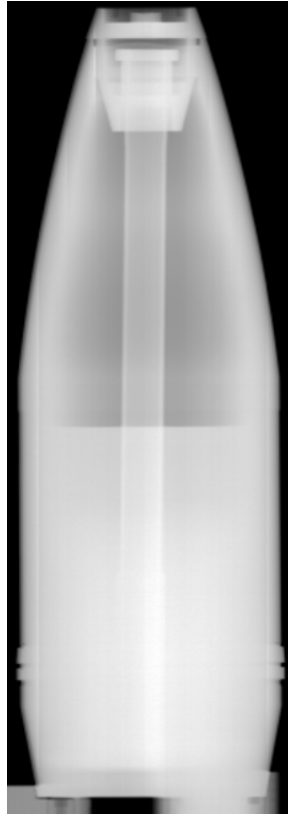
Figure 6. Radiograph of 155-mm munition using fully integrated DT detector. Due to the limited energy of the x-ray generator (300kVp), this image does not appear substantially better than those images acquired with the older detector.
