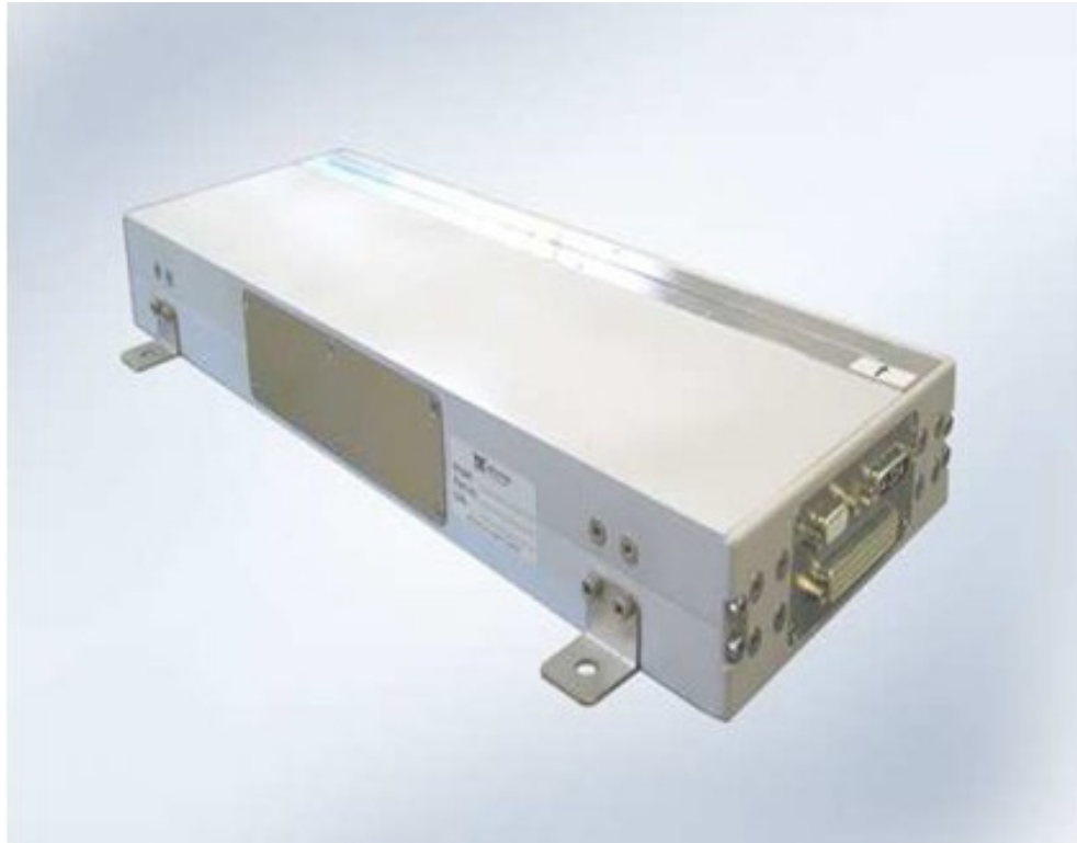
Figure 2. DT linear diode detector array acquired for DRCT single-munitions scanner detector integration task.
