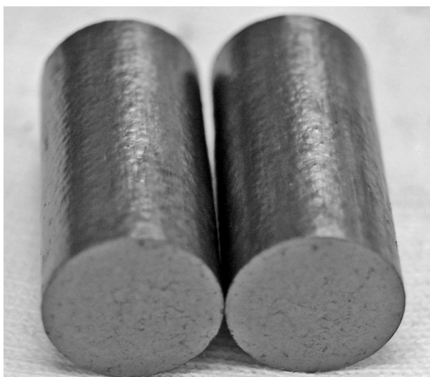
Figure 9. Photograph of heat treated compacts from lot 13064 pressed at 145°C for 220 seconds using proper spray alignment for application of mold release.
