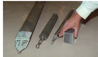
Nuclear fuels are examples of fissionable material. The uranium-aluminum fuels above have a large quantity of U-235.
