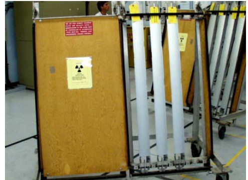
ATR Fuel Transfer Racks include broad base structures and tilted positions.
