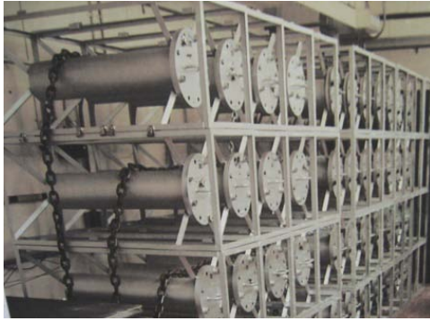
“Birdcage” packages include structure to separate package contents.
