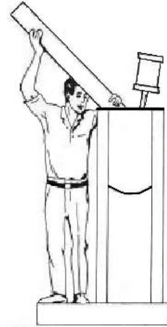
Reconstructed position of worker in 1964 criticality accident, showing the safe-by-geometry cylinder and not-safe-by-geometry tank.
