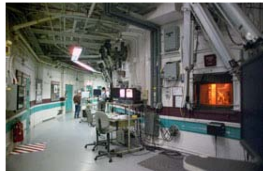
The Fuel Conditioning Facility and Hot Fuel Examination Facility cells have enough shielding to protect personnel in the event of a criticality accident
