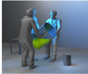
Reconstruction of 1958 criticality accident with human reflectors.
