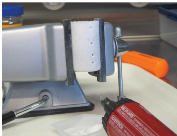
Figure 3.5: Salt sampling technique in the glove box.
