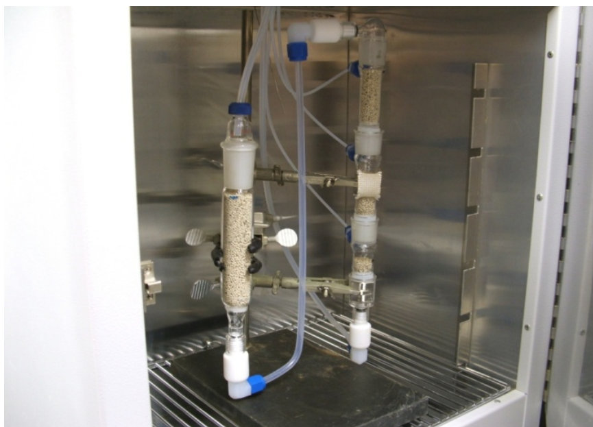
Figure 2-5. Configuration of the sorbent beds inside the temperature-controlled oven.
