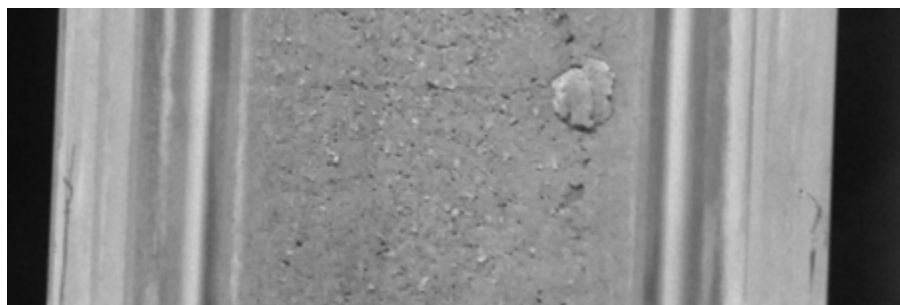
Figure 6. Thick cladding oxide layer with blister damage.
