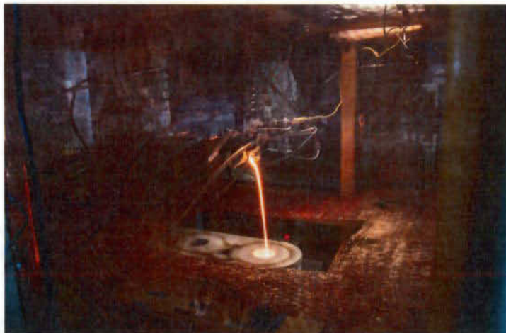
Figure 5. Cold Crucible Induction Melter.
